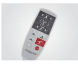
HAND CONTROLLER The possibility of saving positions in the memory (access, examination and ultrasound position) for three doctors – this makes 9 memory positions in total.
